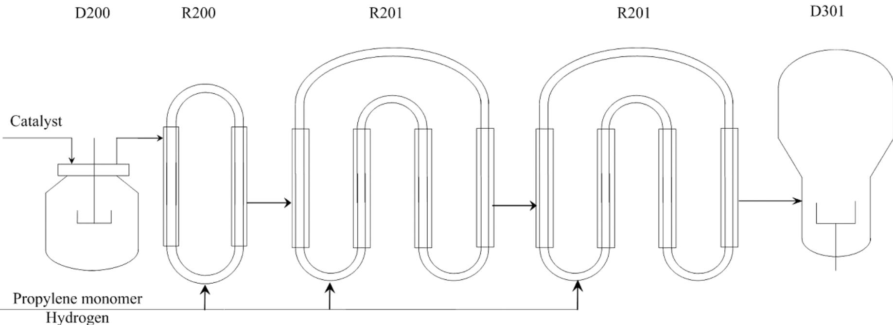
Double-loop liquid propylene polymerization plant of SINOPEC Co. Ltd. (Zhenghai)
