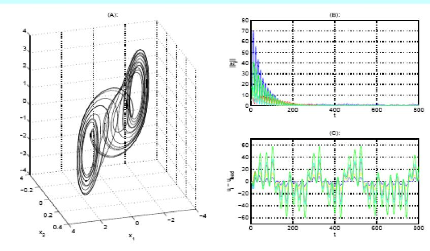
Figure: (A): Phase portrait of leading subsystem, (B):  $||x_i - \overline{x}||$ ,  $\tilde{u}_i = u_i - \overline{u}, i = 1, \dots, 5$ .
