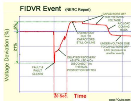
Typical FIDVR Following a 230-kV Transmission Fault in Southern California
