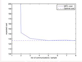
A distributed controller with 100 agents, using only local data. Performance close to optimal centralized controller!
