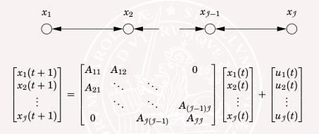
Minimize  $V = \sum_{i=1}^{j} \sum_{t=0}^{N} (|x_i(t)|^2 + |u_i(t)|^2)$ subject to  $x(0) = x^0$  while  $x_i(t) \in X_i$  and  $u_i(t) \in U_i$  for all i, t. (Assume  $X_1 \times X_2 \times \cdots \times X_q$  control invariant.)
