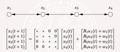
The objective is to make  $\sum_{i} \mathbf{E} |x_i|^2$  small. Can we get a solution where turbines only communicate with neighbors?
