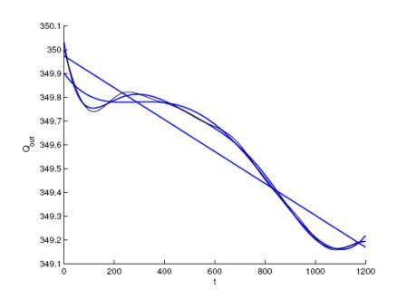
Approximation of typical output water discharge profile (black) by polynomials of degree 1, 4 and 7.
